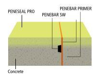
Construction joints: Apply a topical layer of PENETRON crystalline material and/or install PENEBAR SW waterstop between pours.
