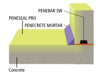
**Cold joints:** A variety of systems can be used here, including PENEBAR SW waterstop (new construction joints) and PENETRON crystalline topical material (existing construction joints).
