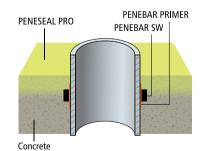
**Penetration:** Install PENEBAR SW waterstop around the penetration.
